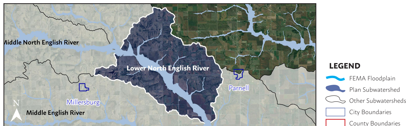
Figure 10. Flood hazard boundary areas for the Lower North English River Subwatershed. Source: FEMA
