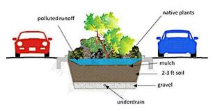
• They generally consist of a permeable liner, a gravel layer, and a planting soil layer on top where plants, shrubs, and trees can be planted.
