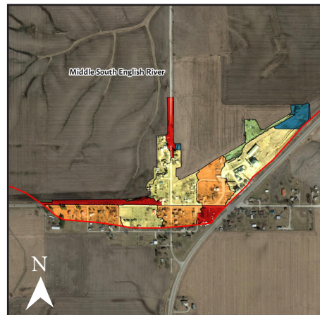
Figure 16. Modeled Phosphorus Load in Webster, IA (lbs/acre/year). Source: UNI GeoTREE
